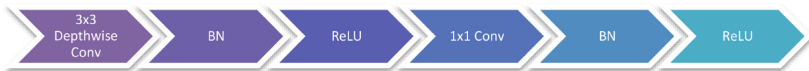
Fig. 13. The flow of depth wise separable convolution (DSC) layer (Goodfellow, Bengio, & Courville, 2016).
